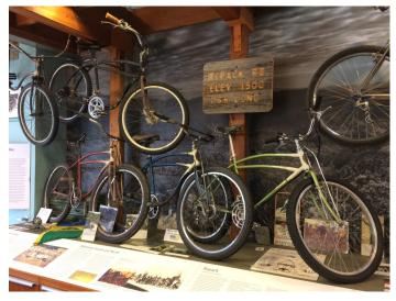
A display of early Repacker bikes. They loved early 1940's Schwinns because of the high bottom brackets, and sturdy frames. They would tear off any extra accessories to make the bikes as light as possible. Riding downhill with only a coaster brake. Later models they added hand brakes, and gears.
