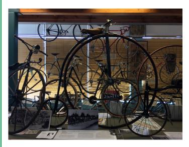
This is one of the larger Ordinary or "Penny Farthing bicycles". The wheel is close to 60" in diameter, so it could only be ridden by someone with 34" long legs! The larger the wheel, the faster these bicycles went. They were prone to flipping forward, causing the rider to take a "header".
